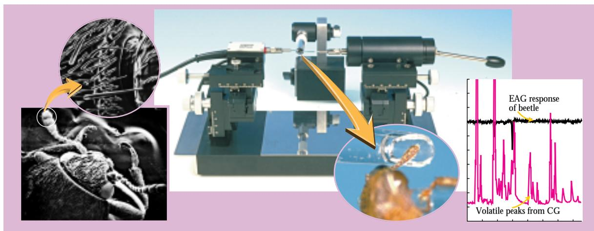
**Figure 4** Raspberry beetle's antennae are covered by olfactory receptors which respond to plant volatiles. Electrical responses to volatiles can be recorded from the antenna using an EAG recording system. A typical EAG is shown; the change in DC voltage is measured in millivolts and is proportional to the odour intensity and number of antennal receptors stimulated by the volatile chemical.
